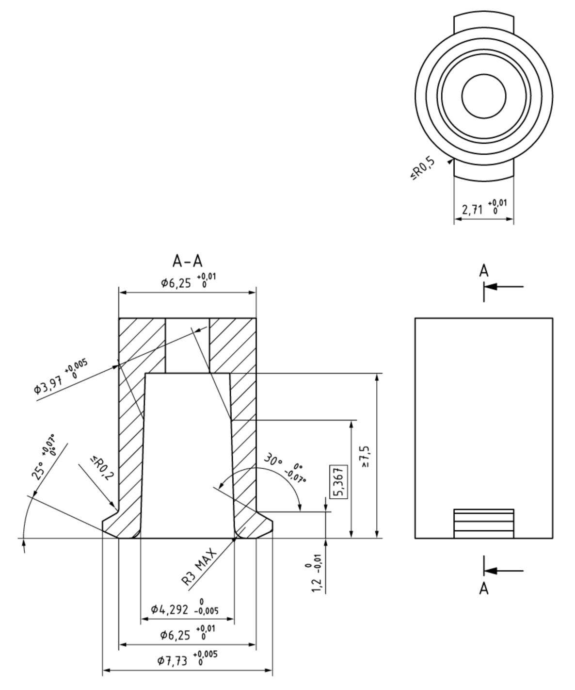
In Figure C.3, all outside edges of lug or thread form shall have a radius between 0,15 mm and 0,20 mm (unless otherwise specified). R may be × 45° chamfer.
