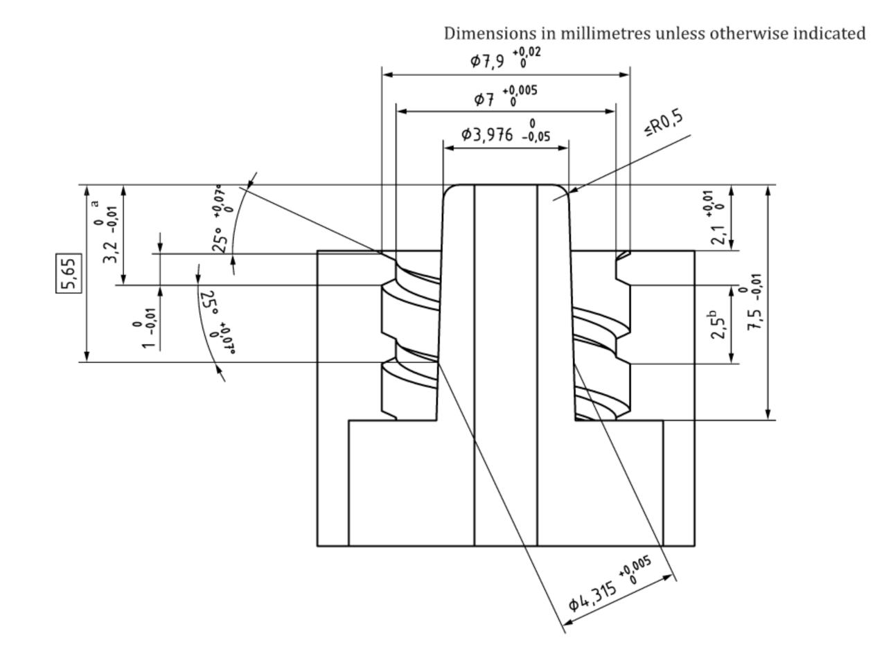
Maximum distance from tip of male LUER LOCK CONNECTOR to the first complete profile of the internal thread
