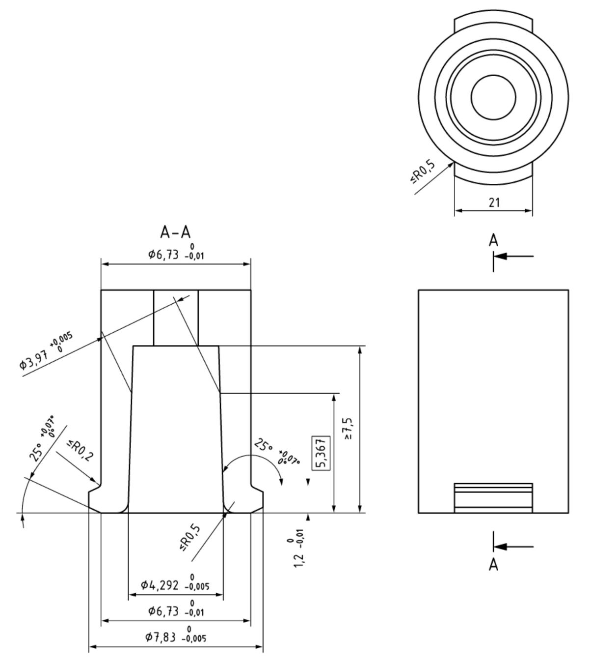
In Figure C.1, all outside edges of lug or thread form shall have a radius between 0,15 mm and 0,20 mm (unless otherwise specified). R may be × 45° chamfer.
