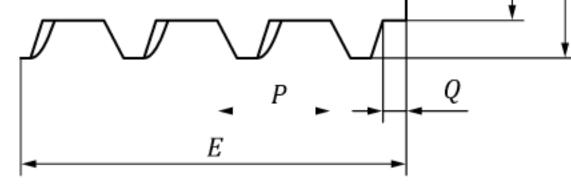
Table B.5 contains the dimensions for this figure. This design and the associated dimensions shall apply to any female LUER LOCK CONNECTOR that has threads in a plane inclined to the axis of the CONNECTOR. There are no dimensional restrictions on thread length. Figure B.6, Figure B.7 and Figure B.8 apply to designs utilizing lugs that are at a right angle to axis of the CONNECTOR.
